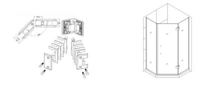
5.Locate the **Support bar (05)**. Adjust the bar to a proper position between **Stationary glass 1(02)** and **Stationary glass 2 (03)**. Level it horizontally. Hold it firmly and outline the bracket's position on the glass. Tighten the setscrews of the support bar and the glass holding screw to secure the glass.
