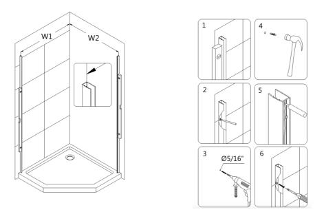
2. Assemble the **U Channel (16)** onto the tile base edge. Drill the holes in the tile base through the holes in the flange of the u channel. Fasten the u channel with the **flat head screw ST4.2×25** (10).
