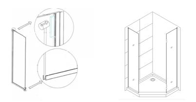
4.Attach the **Hinges (06)** to the **Stationary glass (03)** with the decorative bolts facing inside the shower. Bring the **Glass door (04)** into the Shower base between the two stationary glasses.
