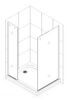
4. Install the **Upper guide rail (03)** to the **Stationary glass (02)** with the **Glass brackets (07)** and tighten the set screws. Slide the **Door stoppers (01)** on each end of the **Upper guide rail** and secure them temporarily. Slide the **Guide Rail brackets (08)** on each end of the **Upper guide rail** and temporarily secure them as well.
