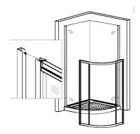
4.Attach the Glass clamp (11) to the glass panel top and bottom (02). Insert the flange antiwater strip (03) into the glass panel (02) and insert the flange anti-water strip (04) on the glass door (05).
