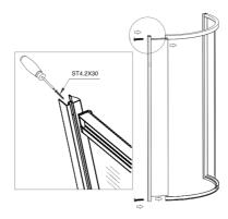
3. Uplift and slide the shower enclosure frame into the groove of the Aluminum wall frame (01)
