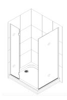
4.Attach the **Hinges (06)** to the **Stationary glass (01)** with the decorative bolts facing inside the shower. Bring the **Glass door (02)** into the Shower base between the two stationary glasses.
